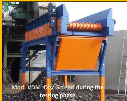
Mod. VDM Disc Screen complete with adjustable substructure
