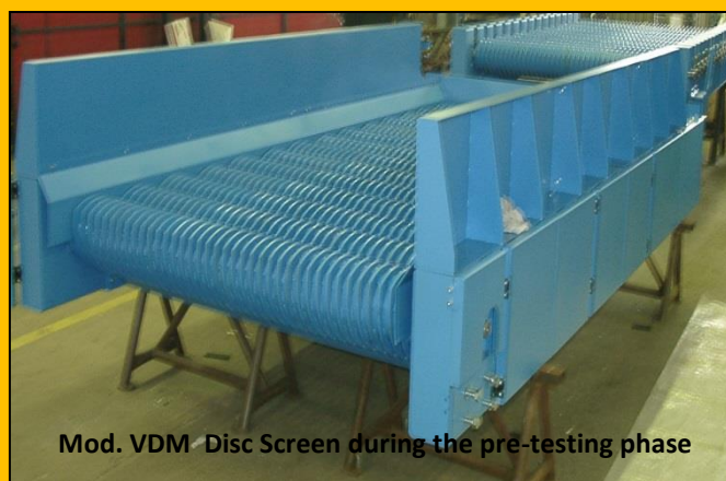
Mod. VDM Disc Screen during the testing phase
