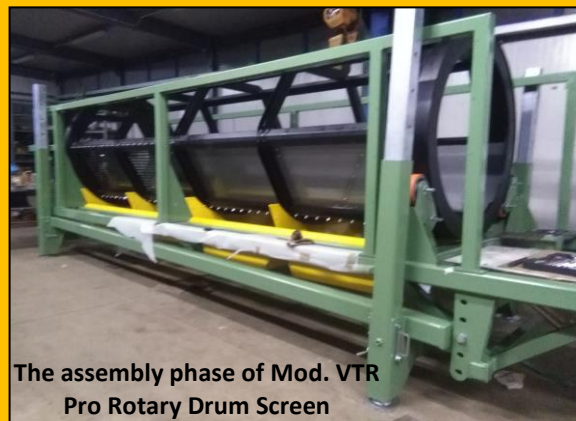
Configuration of the wide-open Mod. VTR Pro Rotary Drum Screen ready for use
