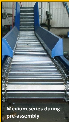
Medium series with heavy belt plus rubber belt and profiles
