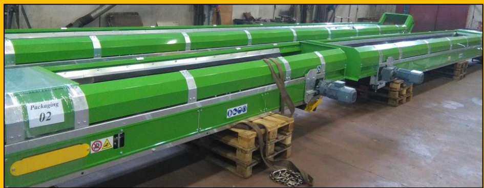
Detail of the flat roll/sliding configuration for the manual sorting
