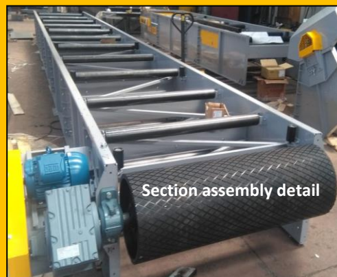
Sidewall Cleat Conveyor Belt during assembly
