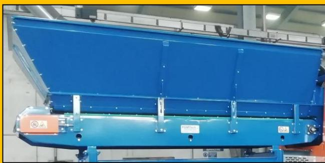
Mod. *TL* Loading Hoppers are designed and built to satisfy the feeding of lines that process medium-light materials without the need for large volumes. This hopper model is mainly used for the feeding of screening and manual sorting systems where there is the constant presence of the operator in charge of loading operations. The Mod. *TL* Loading Hopper is manufactured and customised according to the customer's request in order to completely meet the production needs of the materials processed.
