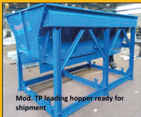
Mod. TP loading hopper of 8.5 cubic meters combined with a 8,500 mm Mod. NB conveyor
