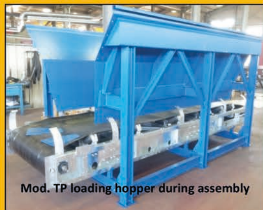
Mod. TP loading hopper of 8.5 cubic meters combined with a 4,600 mm Mod. NB conveyor
